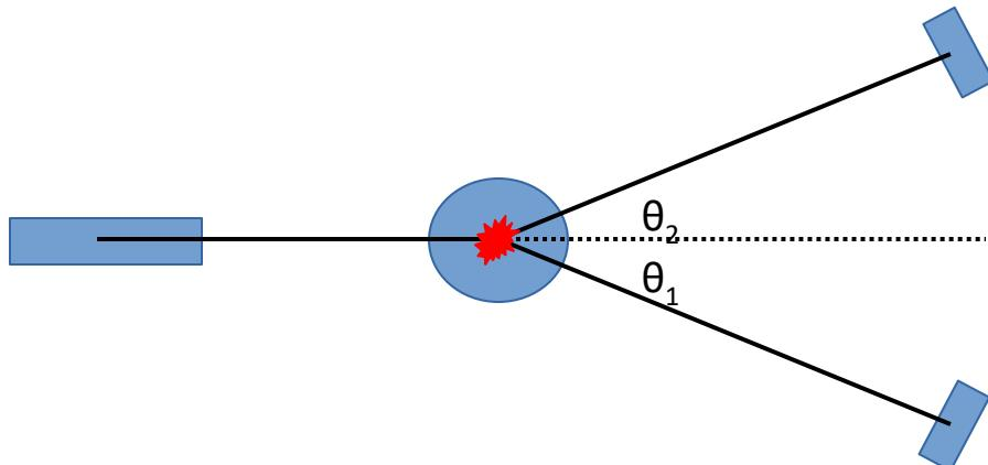
$$\frac{d^5\sigma}{d\Omega_1 d\Omega_2 dS} = \frac{Y_{bu}}{N_n \cdot N_d \cdot \epsilon(E_1) \cdot \epsilon(E_2) \cdot \alpha(E_0) \cdot \alpha(E_1) \cdot \alpha(E_2) \cdot d\Omega_1 \cdot d\Omega_2 \cdot dS}$$
