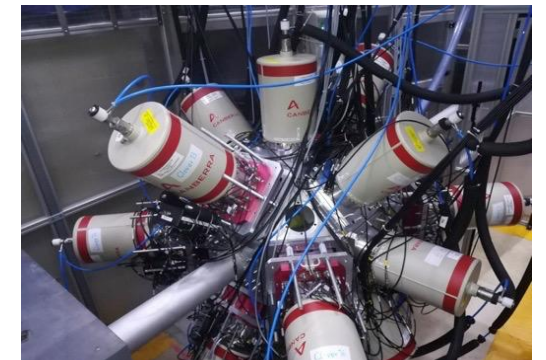
16 HPGe clovers (8 from IFIN-HH) high resolution and efficiency \gamma detector array
